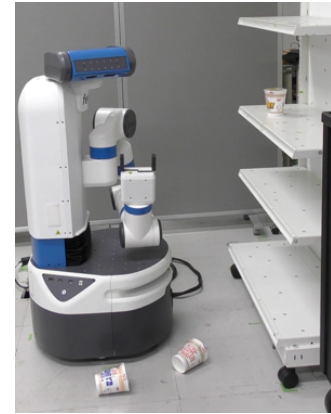
Fig. 9: Demonstration setup emulating a convenience store shelf, comprises a Fetch Robot, a shelf and three types of Noodle Cups. In the proposed scenario, two cups have fallen on the ground, in an unknown pose, due to a customer action.
